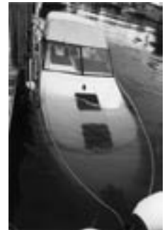
This boat filled with water and sank because the scuppers were clogged with leaves.
